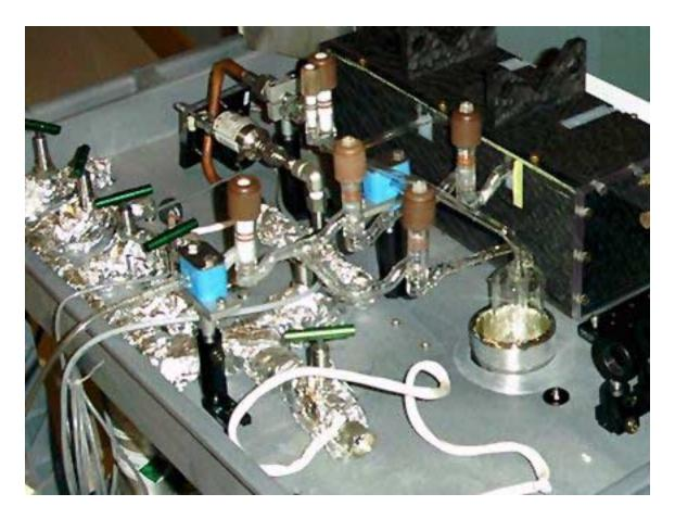
Figure III.3. Freeze cell and manifold of human inhalation cart. This close-up shows the metal and glass manifold, as well as the covered pump cell. The dewar surrounding the freeze cell is partially lowered to make the freeze cell visible.
