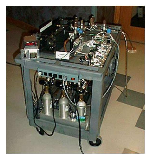
Figure III.1. Front of human inhalation cart. Xe,  $N_2$ , and He cylinders are visible, as are the temperature and pressure gauges. The oven surrounding the pump cell (black casing on left side of cart) has been opened to provide a view of the pump cell. A small inhalation bag mated to the cart outlet is visible on the right side.
