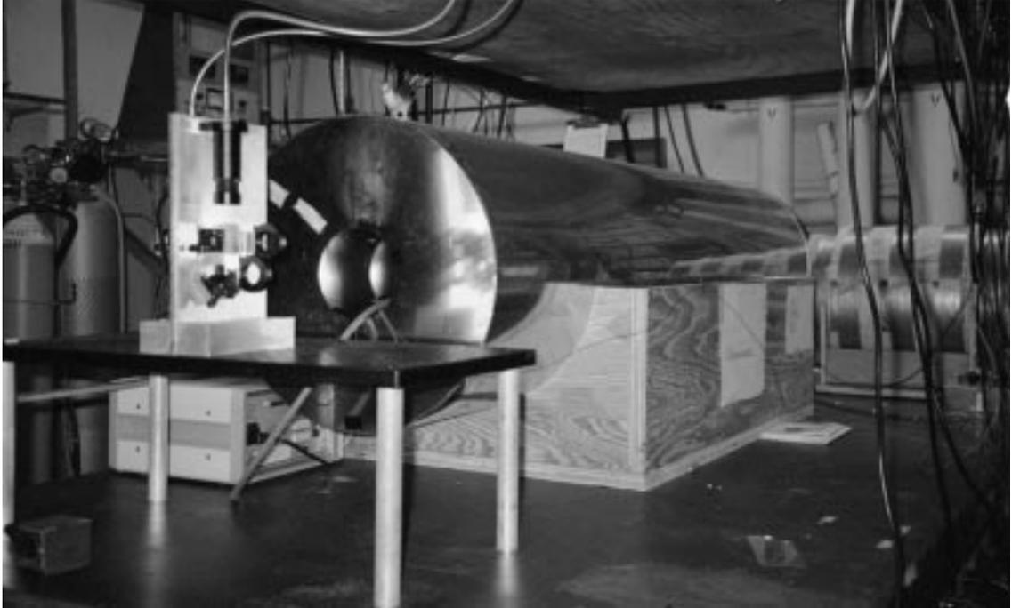
Figure 3.15: A photograph of the LDA optical fiber, collimating lenses,  $\lambda/4$  plates, and polarizing beam splitter cube used in the DNGM experiment. The optical setup is situated approximately 1 foot from the end of the outer  $\mu$ -metal shield.
