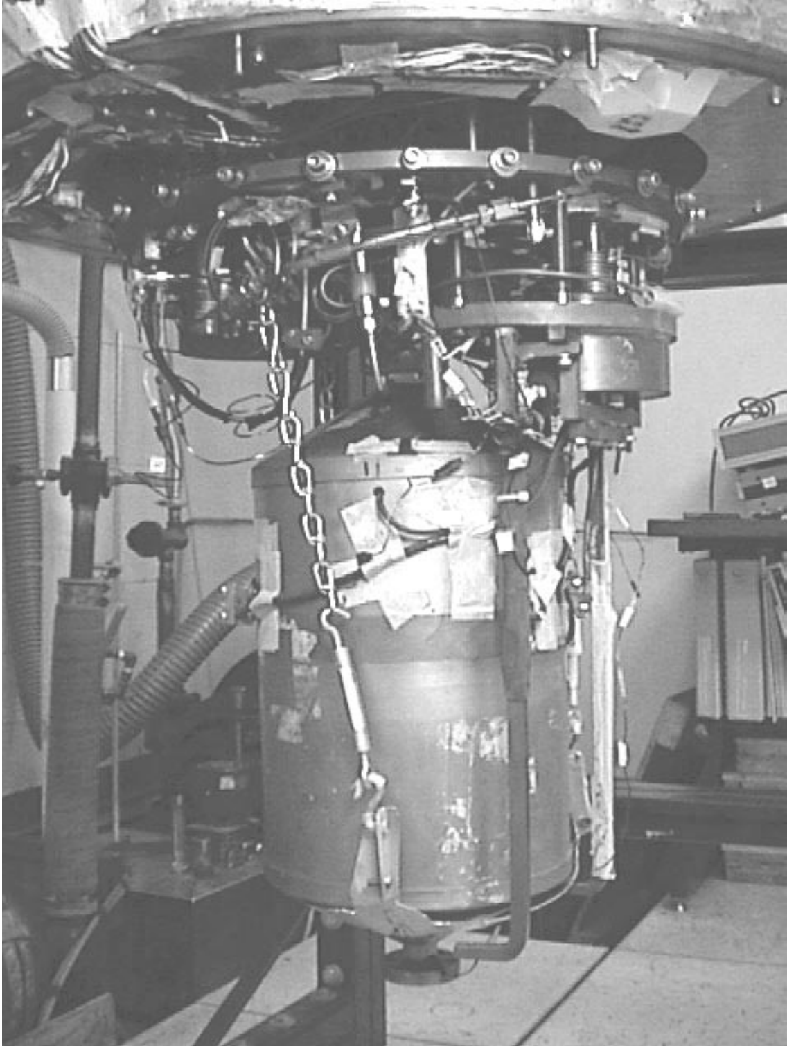
Figure 5.12: Cryostat and maser. At the top is the 77 K jacket (77 K shield not mounted). Below this is the perimeter of the 2K plate (without the 2K shield). The ^4\text{He} pot is at the left, the ^3\text{He} pot is to the right, and the maser's outermost magnetic shield is at center.
