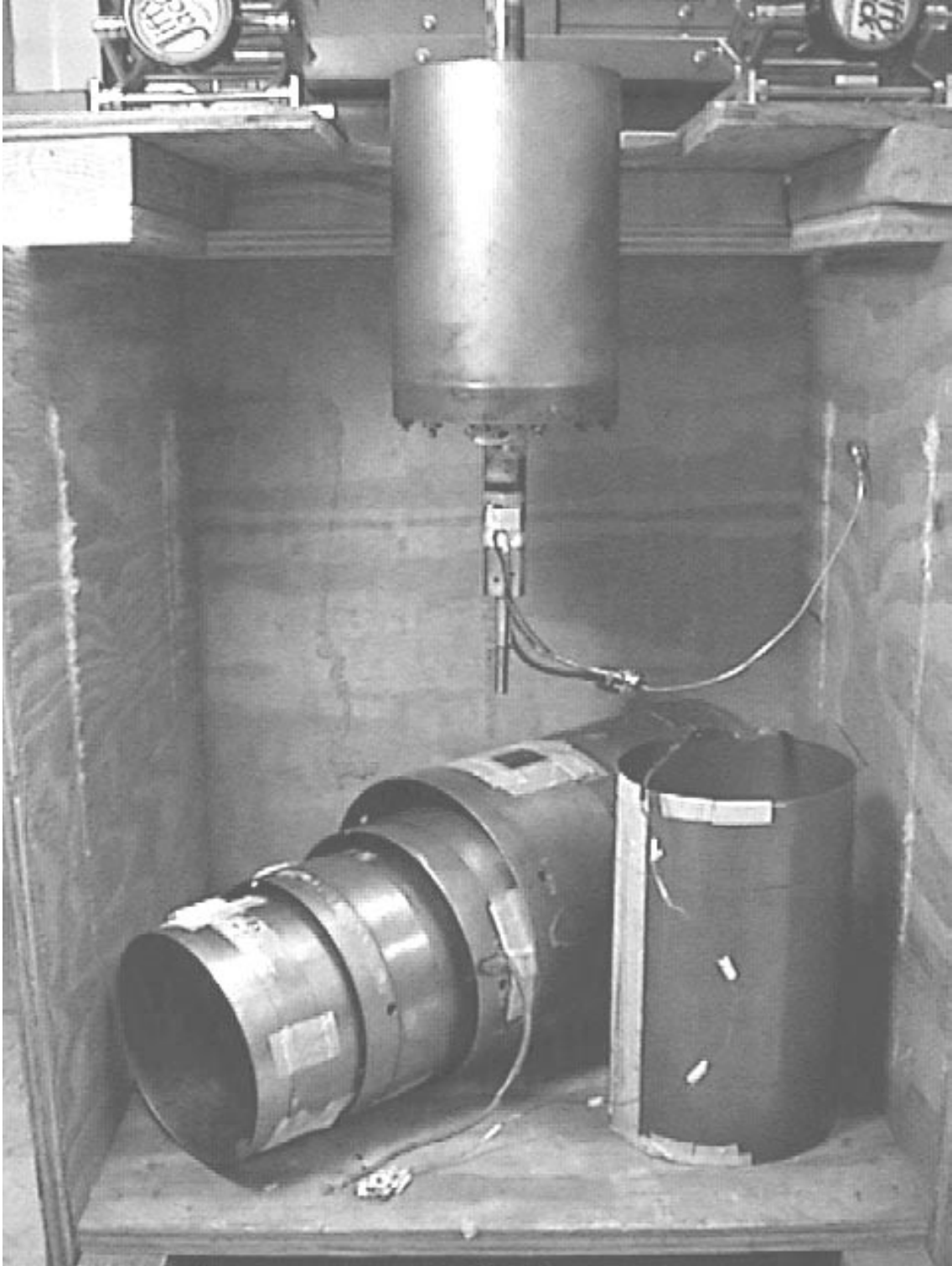
Figure 5.8: Copper pot containing cryomaser cavity (top), magnetic shields (left), and solenoid (right).
