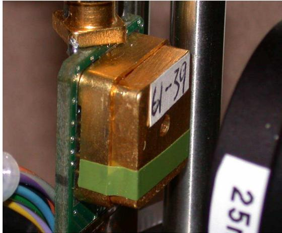
Figure 3.1: A VCSEL from Kernco. Dimensions are about 1.5 cm by 1.5 cm by 0.5 cm.
