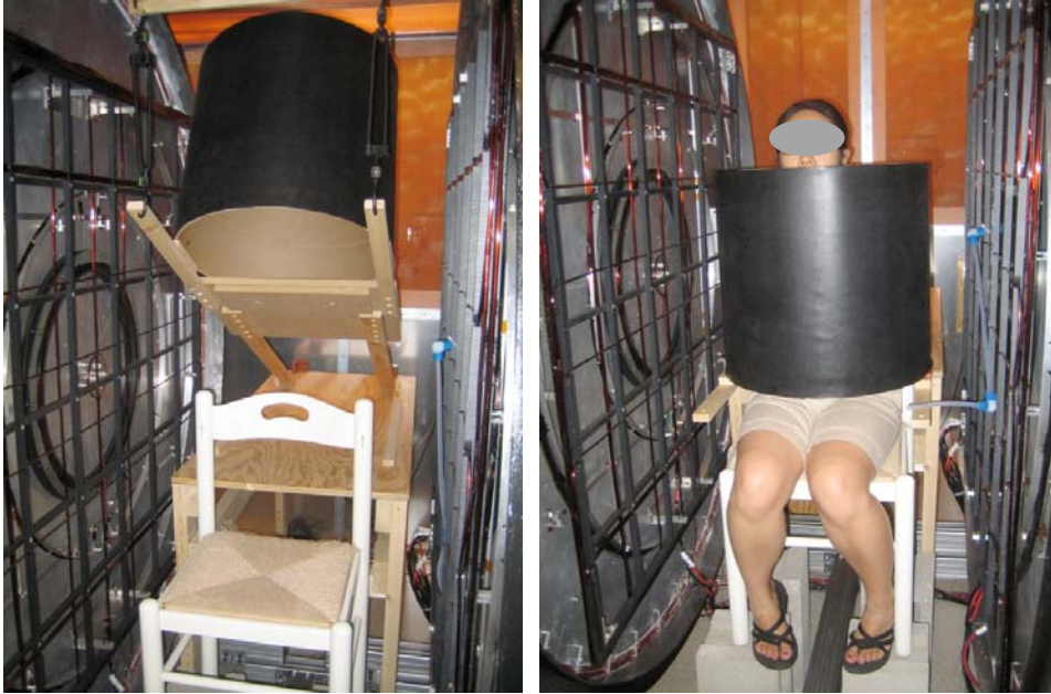
Figure 3.29: Left: The arrangement for upright imaging, with the RF coil locked in the upper position for subject access. Right: The RF coil in place with a subject in the upright orientation.
