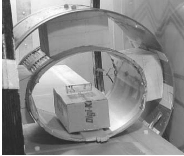
Figure B.5: Photograph of the transmit and receive coils for the open-access human MRI system. The large Helmholtz transmit coil was bolted onto the subject imaging table, and the receive coil was attached using foam spacers and plastic bolts.
