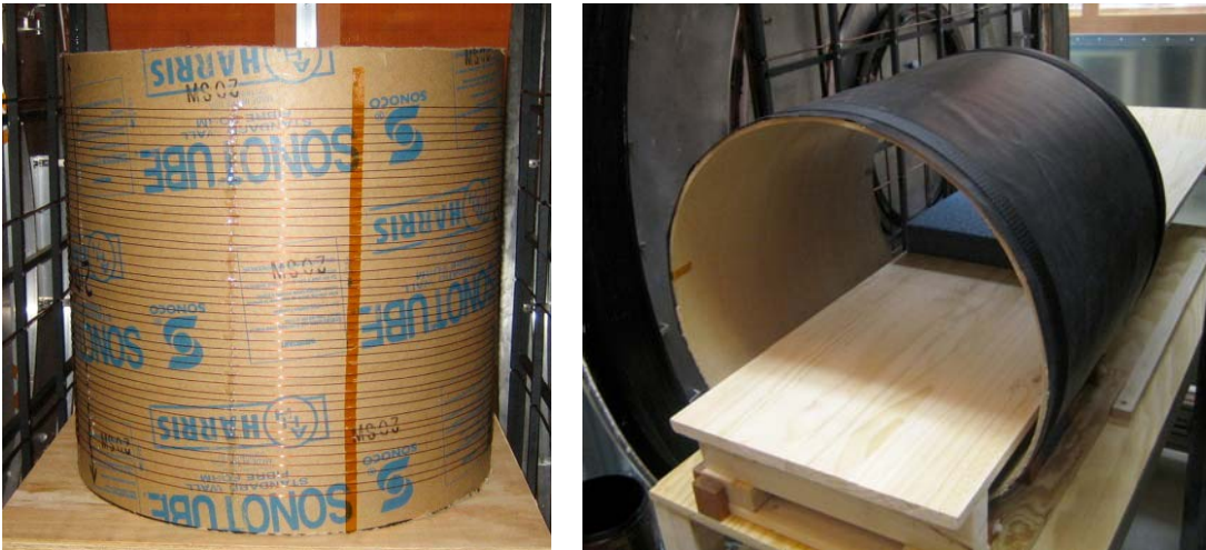
Figure 3.20: Left: A photograph of the human chest coil showing the winding pattern and cardboard cylinder form. Right: The completed human chest coil wrapped in rubber insulation and mounted on the subject table.
