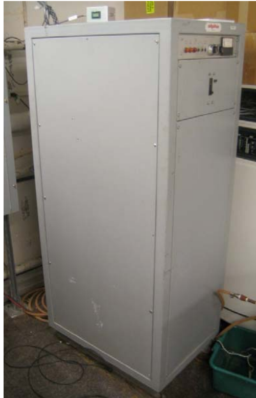
Figure 3.5: A photograph of the B_0 power supply. The small box at the top is the digital voltmeter we use to obtain a high-precision measurement of the output current (high-current resistor not shown).
