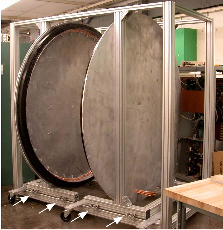
Figure 3.4: A photograph showing the aluminum frame of the LFI and the two aluminum flanges. We wound the outer B_0 coil onto the frame prior to attaching the flange to the frame. The arrows at the bottom show the location of the Delrin pads on which the flange and its stand rests. We used detachable casters to transport the entire frame to its final location; they were later removed.
