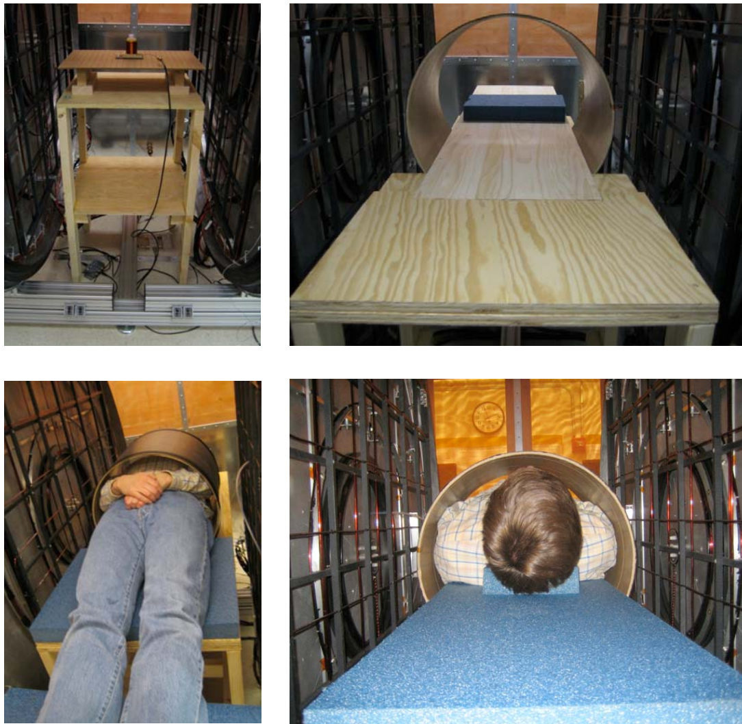
Figure 3.28: Clockwise from upper left: A wooden stand for NMR phantom studies. Fully assembled subject table with the human chest coil installed viewed from the -x side. Supine subject with chest coil in place, viewed from +x side. Same subject with chest coil in place, viewed from the +x side.
