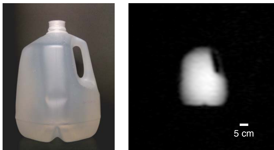
Figure 4.3: Photograph and corresponding projection MRI of a 3.8 L water jug. Imaging parameters: B_0 = 65 G, \omega_0 = 275 kHz, 128 \times 64 ( z, y ) zero-filled to 128 \times 128 , FOV = 60 cm, 8 signal averages, T_R = 3 s, T_E = 10 ms, total scan time \sim 26 minutes. The image shows both the thin water-filled handle of the jug as well as the dimple across the bottom of the container. The image resolution is 4.7 mm.
