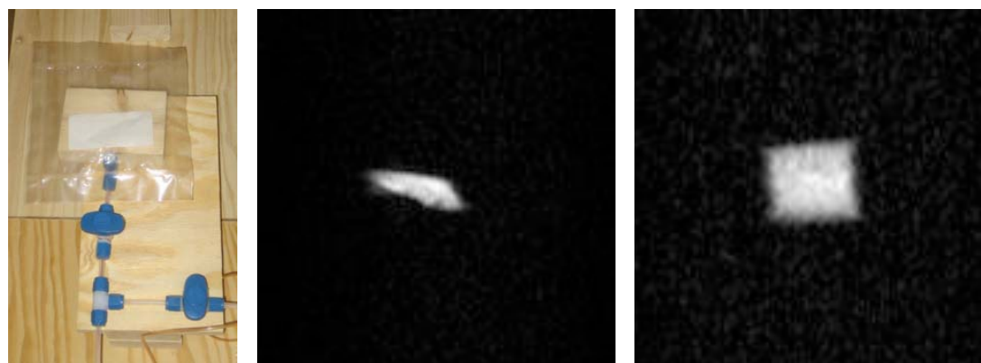
Figure 4.13: Left: a photograph of the 500 cc Tedlar bag with gas delivery tubes in place. Middle and Right: Two sample xz projection images of the Tedlar bag with the bag oriented along the yz and xz planes, respectively. Imaging parameters: B_0 = 65 G, \omega_0 = 210 kHz, 128 \times 64 , zero-filled to 128 \times 128 , FOV = 50 cm, no signal averaging, \theta = 3^\circ , T_R = 120 ms, T_E = 10 ms, total scan time \sim 7.7 s. SNR \sim 30 –60.
