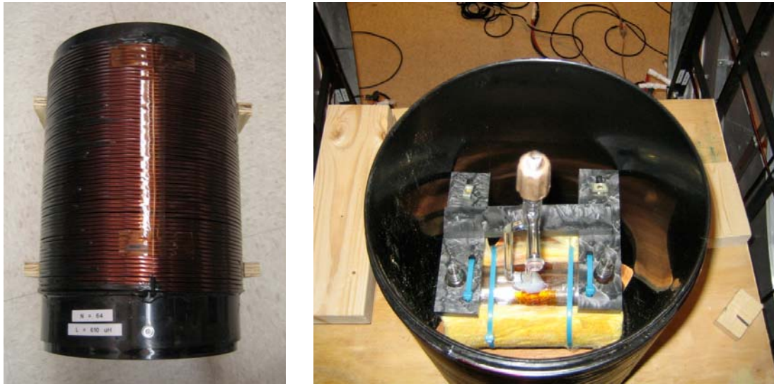
Figure 3.19: Left: A photograph of the 25 cm-diameter general-purpose RF coil used in several ^3\text{He} and ^1\text{H} experiments, including human head imaging. Right: a photograph of the coil oriented along the y axis, with a ^3\text{He} cell inside.
