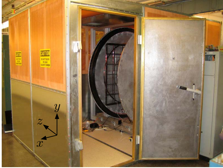
Figure 3.24: A photograph of the Faraday cage with the entrance door open. The -z and +x corner of the LFI magnet is closest to the doorway. Axes are labeled.
