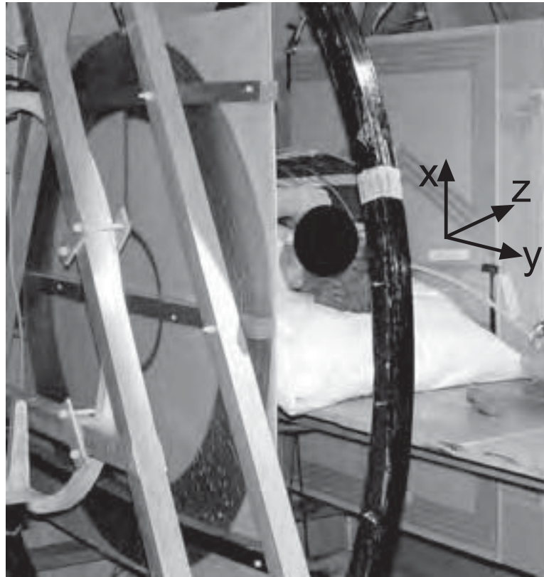
Figure B.4: The planar gradient sets mounted on the aluminum support frame of the open-access human MRI B_0 coil system. The x and y gradients are placed just inside of the z gradients, relative to the subject (seen in supine position). As such the z -axis gradient is visible on the subject's left, and the x -axis gradient is seen to his right.
