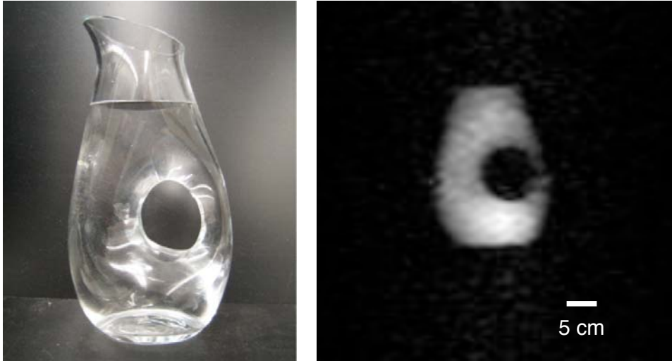
Figure 4.1: Left: a photograph of a glass pitcher partially filled with water. Right: ^1\text{H} image of the pitcher obtained with the LFI, using the 25 cm-diameter coil. Both the coil and the pitcher are oriented vertically ( y ). Imaging parameters: B_0 = 50 G, \omega_0 = 210 kHz, 128 \times 64 ( z, y ) zero-filled to 128 \times 128 , FOV = 50 cm, 9 signal averages, T_R = 3 s, T_E = 10 ms, total scan time \sim 32 minutes. The maximum SNR \sim 50 for this projection image.
