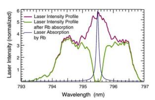
Fig. 1 Laser line-shape from a typical LDA commonly used for spinexchange optical pumping. The pink line is the measured laser output, the green line is the laser spectrum after travelling through an optical pumping cell. The blue line is the calculated laser absorption by rubidium in the spinexchange process, for common 129Xe operating parameters.
