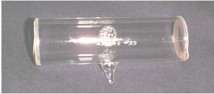
Figure 2.10: Natural abundance Rb vacuum cell (no buffer gas, uncoated walls). Length is 7.5 cm and diameter is 2.5 cm. Metallic Rb can be seen in the center. The cell is resting on J. Vanier and C. Audoin, The Quantum Physics of Atomic Frequency Standards , Institute of Physics Publishing (1989).
