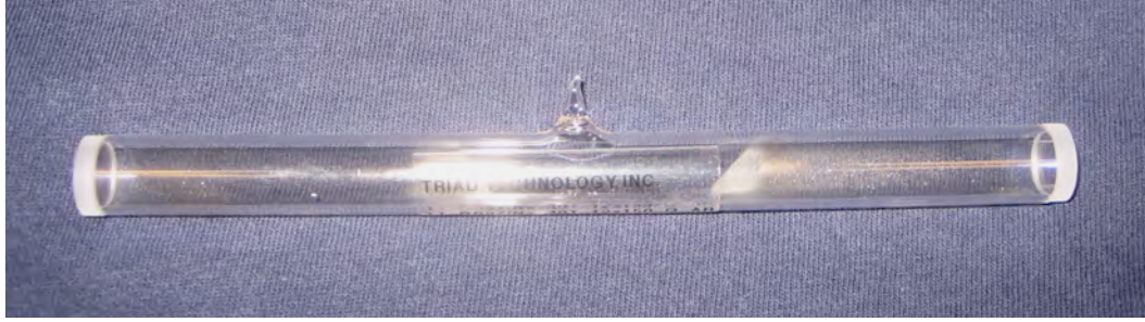
Figure 4.2: The long, narrow Rb vapor cell used in stored light optimization experiments to mitigate the effects of radiation trapping. Length is 15 cm and diameter is 1.2 cm.
