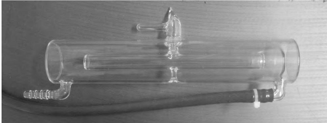
Figure A.6: Double-jacketed, long, narrow coated Rb vapor cell. The surrounding chamber served as an oven for applying the paraffin wall coating, and for operating optics experiments.
