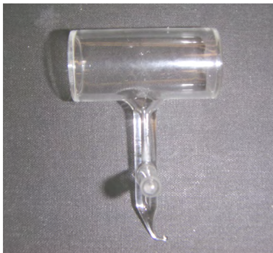
Figure 2.8: A paraffin-coated vapor cell. Length is 5 cm and diameter is 2.5 cm. Note the sidearm (pointing out of the page), branched out of the main cylindrical cell body, as a way to store Rb metal, keeping it from sticking to the coated walls.
