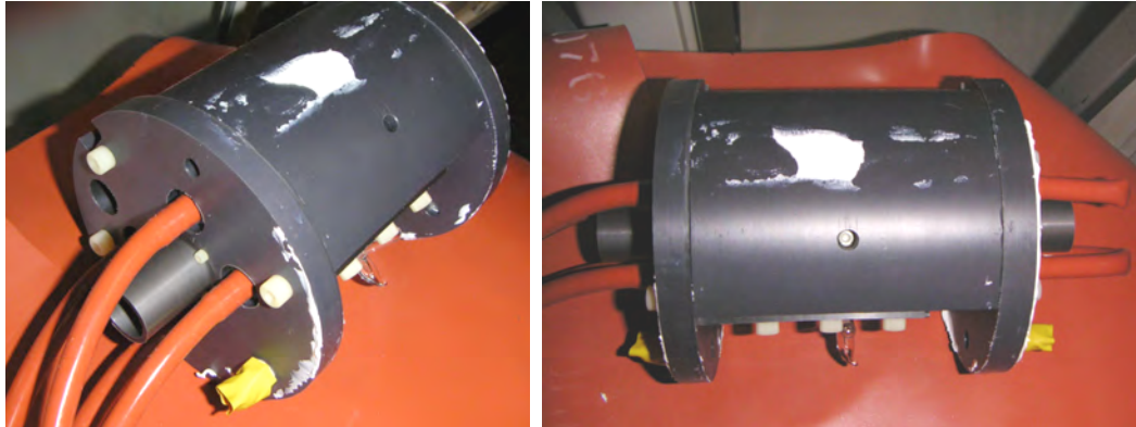
Figure 2.6: The cylindrical Nylatron oven used for heating Rb vapor cells. Note the Rb arm sticking out the bottom, done this way to maintain the Rb at a lower temperature in wall-coated cells.
