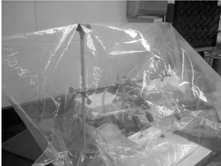
Figure A.4: “AtmosBag” used to provide a nitrogen environment for opening a ^{87}\text{Rb} metal container and transferring the ampule to the cell manifold. Shown here for a manifold with three miniature cells.
