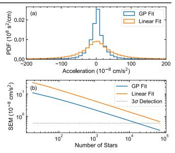
FIG. 3. (a) Probability density function (PDF) of fitted stellar accelerations for  $\sim 7.5 \times 10^4$  stars using Gaussian processes (GP) (blue) and a simple linear fit (orange). 60 cm/s of white noise and quasiperiodic correlated noise ranging from 50 to 250 cm/s is added to each time series. (b) Standard error of the mean (SEM) vs number of stars observed. A  $3\sigma$  detection (dotted gray line) is obtained after about  $2 \times 10^4$  stars for the GP fit.
