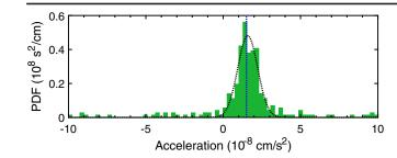
FIG. 4. Probability density function of fitted stellar accelerations for  $10^3$  stars, using a simple linear fit and filtering using periodogram power. The only source of noise included is 10 cm/s white noise. The dotted black curve is a Gaussian fit to the histogram (a guide to the eye). The injected acceleration signal of  $1.5 \times 10^{-8} \text{ cm/s}^2$  is shown as a blue dotted line.
