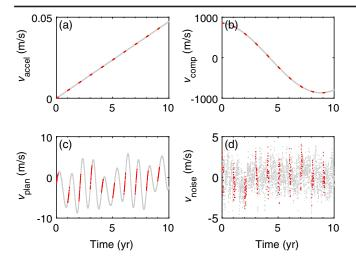
FIG. 2. Example of a synthesized RV time series for a single primary star, showing the four contributing mechanisms considered in our analysis. The effects of (a) the acceleration due to the Milky Way gravitational potential, (b) stellar companions, (c) planets (multiple planets in this case), and (d) "noise" including stellar activity and instrumental effects are depicted. Red dots are the observed nights and gray dots represent all nights.
